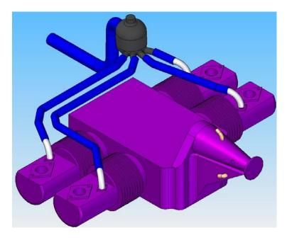
20. 1) Loosen the Bent Socket screws from cylinder N°4 and rotate the curve about 30 °. Connect hoses are as follows
