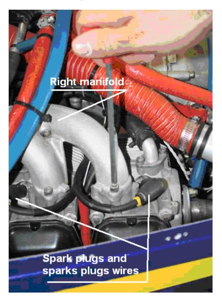
CAUTION: once removed the manifold of the engine, plug the holes input cylinders
