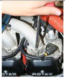
7) Remove the electronic ignition box (Coil Assembly Module).
