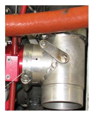
The hot air selector is fixed to the carburettor with a clamp of 27 to 61 mm
